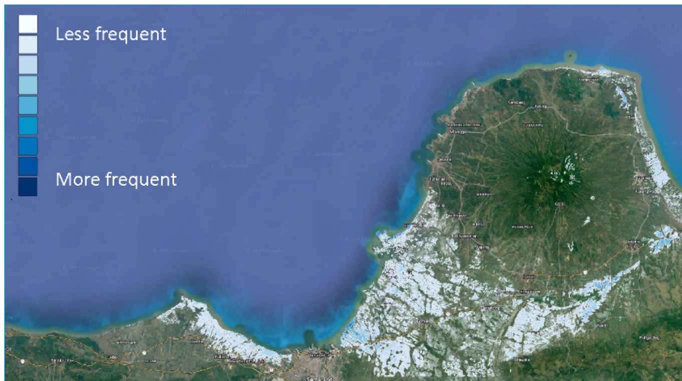
Figure 18. Flood frequency in Surabaya (Indonesia) darker colours depict areas that have been flooded more frequently in the monitoring period here from 2015 to 2023, processed by LIST/CIMA/Wasdi Sarli).
