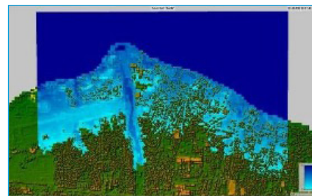
Figure 27. Plan view of DTM + Buildings, Dili with 10 m flood
