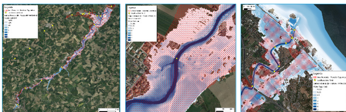
Figure 22. Maximum Flood Water depths in the Misa River (Marche Region, Italy) in the immediate aftermath of the event that took place from 15 to 16 September 2022. The figures show a comparison of the TELEMAC-2D (blue scale) with the flooded area as detected by Copernicus-EMS (Sentinel-1, Cosmo-SkyMED, in red) synoptic view and 2 details. Courtesy of CIMA Foundation.
